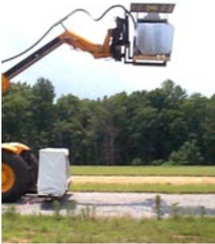
Figure 1. Downward looking laser Doppler vibrometer (LDV) based acoustic-to-seismic coupling landmine detection system in a field environment. The LDV head is mounted on a vehicle 3.5 meters above the ground. The laser beam is focused downwards onto the ground surface. Two loudspeakers in front of the vehicle wheels radiate acoustic waves towards the road surface.
