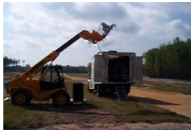
Figure 4. Forward-looking laser Doppler vibrometer based acoustic-to-seismic coupling landmine detection system in field environment. The laser beam is focused forwards onto the middle of the road shown on the right side of the photo.
